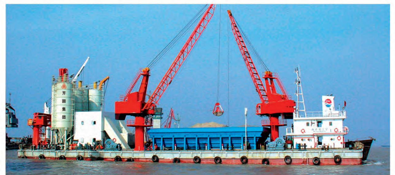
▲ Shipborne mixing plant
