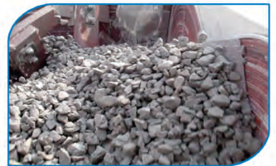
Test running with 10% overloaded dry aggregate
