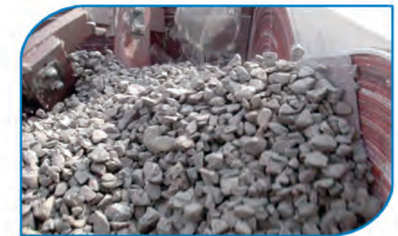
Test running with 10% overloaded dry aggregate
