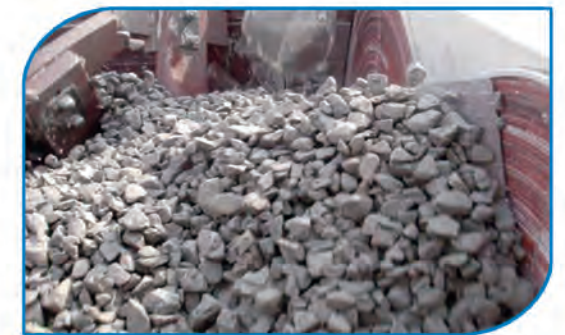
Test running with 10% overloaded dry aggregate
