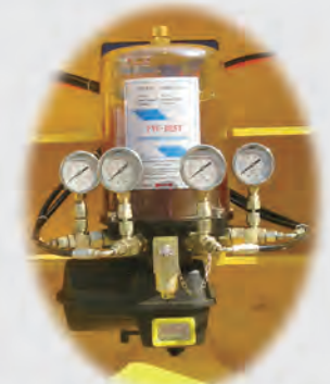
Centralized lubrication with shaft-end pressure monitoring
